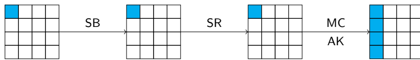
Figure 5.2: Visual illustration of how the fault propagates when a fault is injected at the beginning of one AES round (not the last round) in byte s_{00} . Blue squares correspond to bytes that can be affected by the fault.
